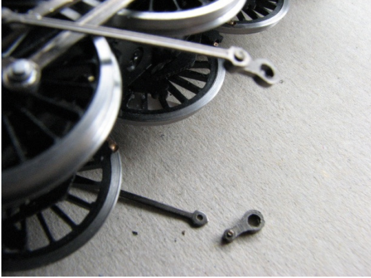
Return crank separated from lower rod.
