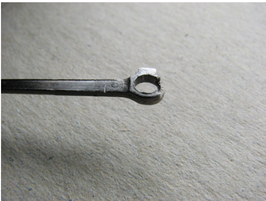
Connecting rod showing the “lump” that needs removing.
