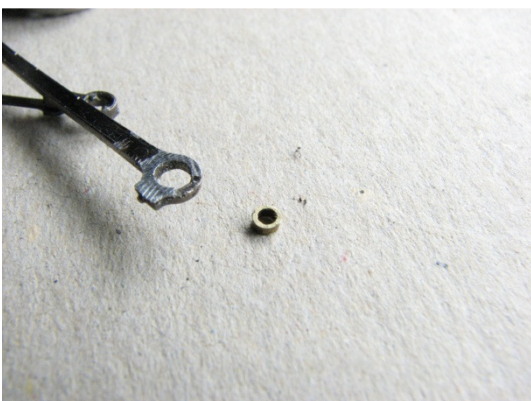
Modified connecting rod plus bush cut from brass tube.
