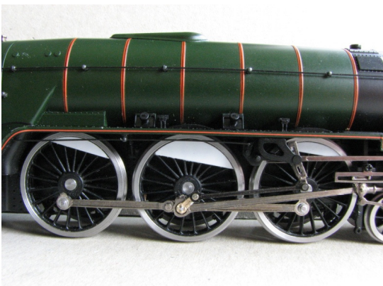
Completed valve gear.
